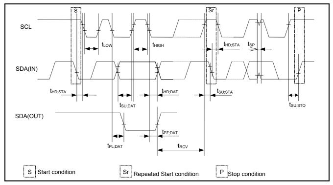
Caution: When accessing this device, all communication from transmitting the start condition to transmitting the stop condition after access should be completed within 0.5 seconds.
