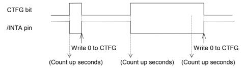
Note: When using the clock precision adjustment function, the periodic interrupt's cycle changes once every 20 seconds.
